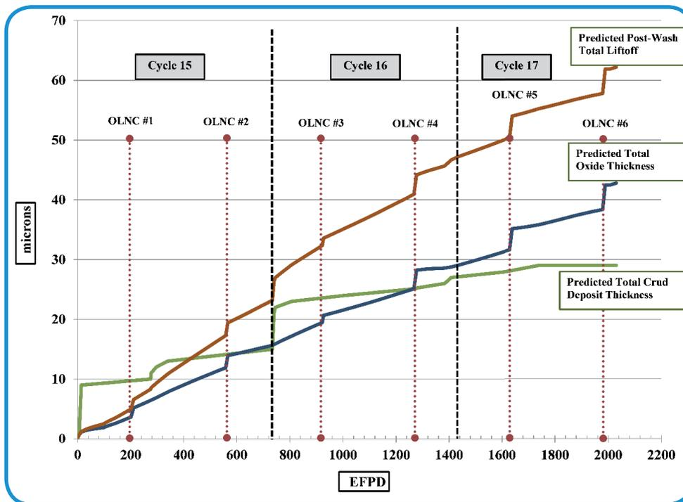
Figure 1: Predicted Post-Washing Total Liftoff Predictions at Crud Induced Localized Corrosion (CILC) Limiting Core Location
