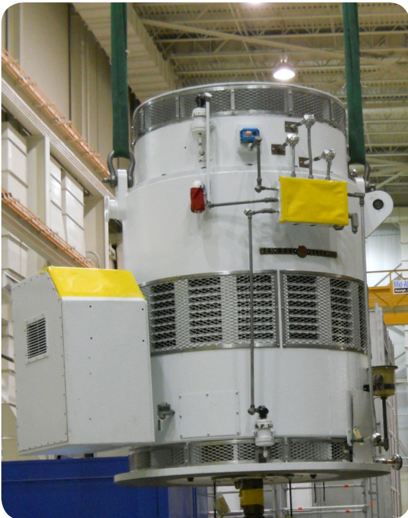
GE BWR Recirc Motor after Refurbishment
