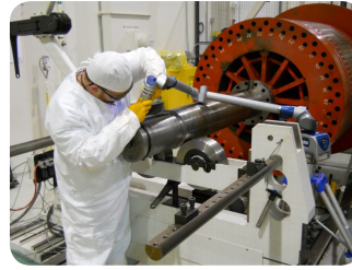
Measurement of Rotor from Allis Chalmers RCP
