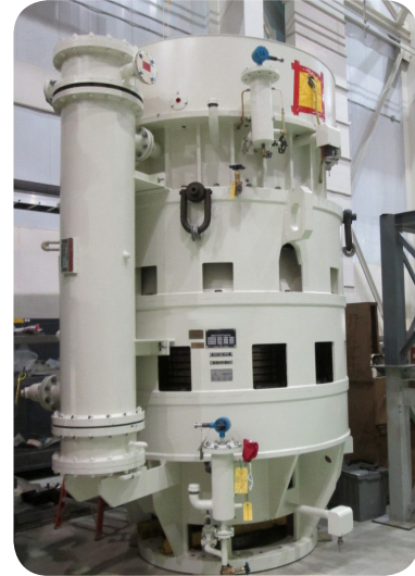
Westinghouse PWR RCP Motor
