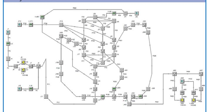
Figure 2: BWR reactor recirculation and residual heat removal (RHR) systems
