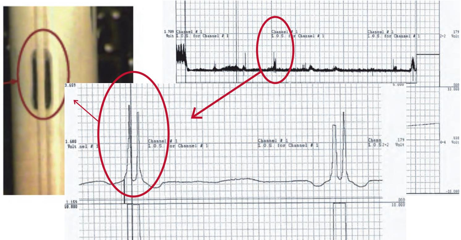
Example of an HTP™ Wear Scar and associated data Acquisition
