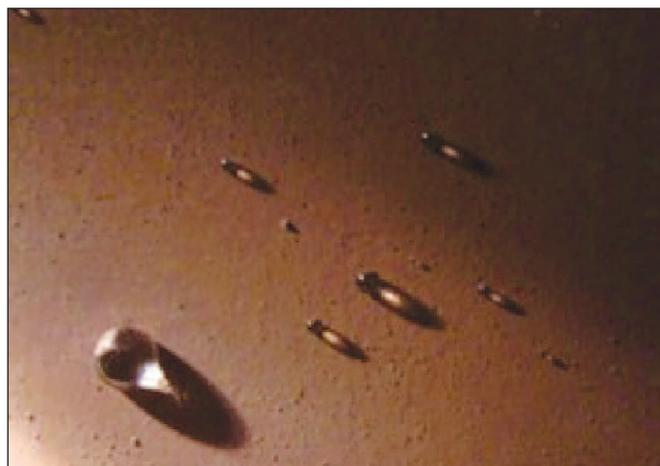
Figure 2: Water droplet testing during visual inspection in the condenser of a NPP during an outage following time-limited FFA application [5].
