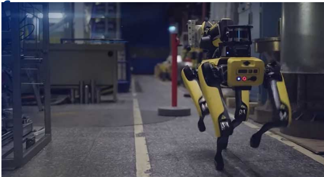
Demonstration of an agile and mobile robot used for doing radiological measurements and documentation.
