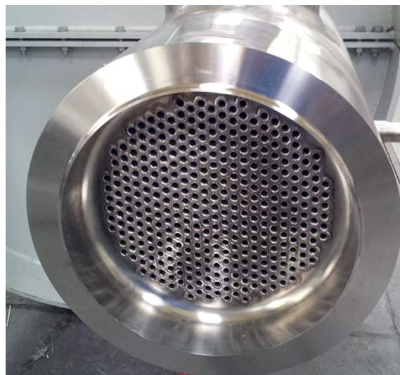
One of two tube sheets of hairpin heat exchanger for Volume Control System
