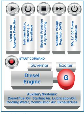
Modular Control Concept: Standard interfaces allow easy system configuration, integration and commissioning
