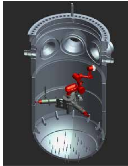
Flip joint to allow vessel weld examination with arm either above or below the base
