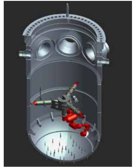
Full access near radial supports and meridional welds without re-positioning base
