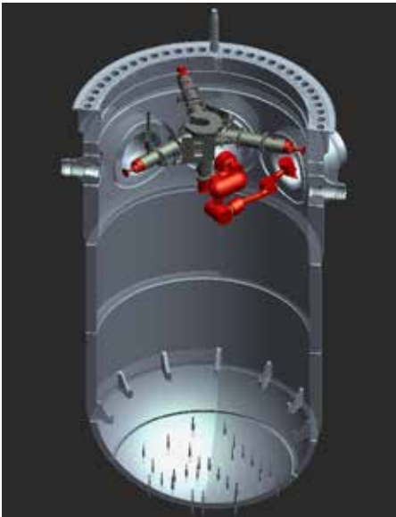
Kinematics optimized for “rainbow” scans around nozzles
