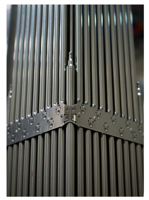
The innovative 11 x 11 rod array design increases tolerance for pellet-clad interaction. That means you can maneuver assemblies faster, and your plant can operate at a higher capacity factor.
