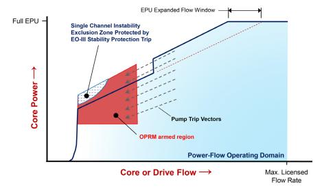
A small scram-protected exclusion zone, well out of the normal power-flow operating domain, allows continued use of the original Option III Detect & Suppress stability solution for extended flow window operations at EPU.
