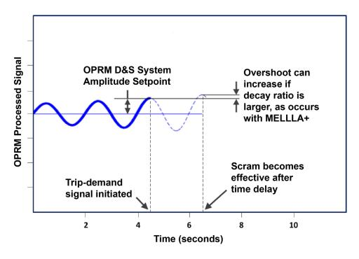
EO-III methodology allows continued use of the OPRM hardware and software without change, addressing more severe instability conditions through a simple power uncertainty factor applied to the Hot Channel Oscillation Magnitude used in the setpoint analyses.
