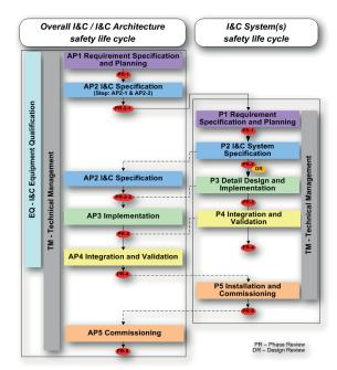
Connections between the overall I&C safety life cycle and the safety life cycles of the individual I&C systems – following EC 61513 (2011)
