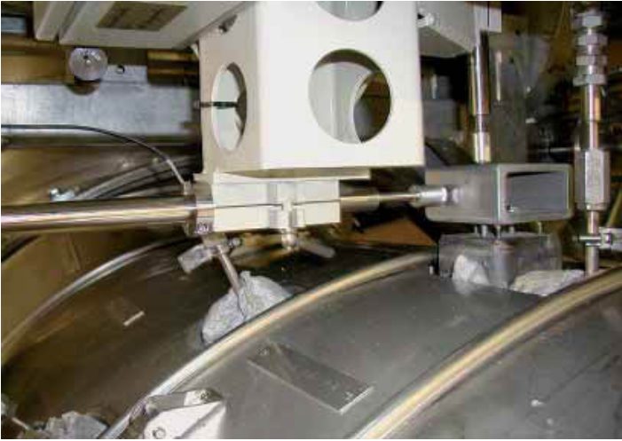
Special relative displacement sensors for measuring loop vibrations and quasi-static loop displacements
