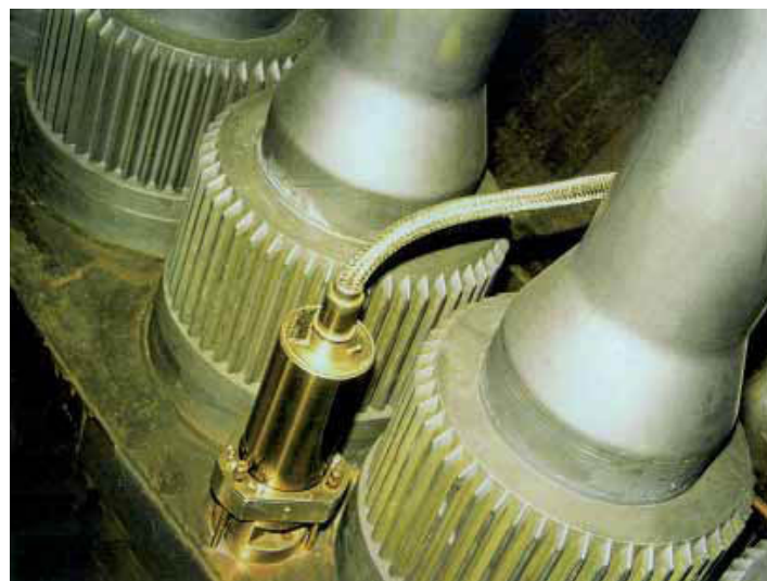
Special high-sensitive absolute displacement sensor for applications in harsh environments (measuring RPV vibrations at closure head)
