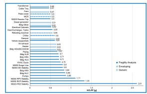
One of the results of SMA (exemplary): ranking of structures/components, from weakest (transformer) to strongest (pressurizer)
