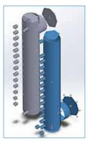
3D scan of the original coil header which was used to pull dimensions and generate fabrication drawings.
