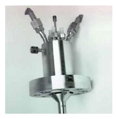
Flange version of the high-temperature reference electrode
