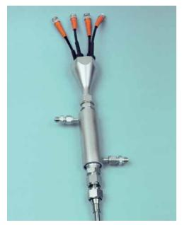
Laboratory version of the high-temperature reference electrode
