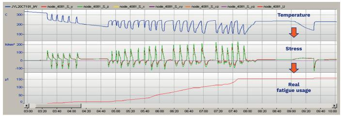
Example of a thermal power plant: measured load history like temperature → precise stress history → precise damage and CUF
