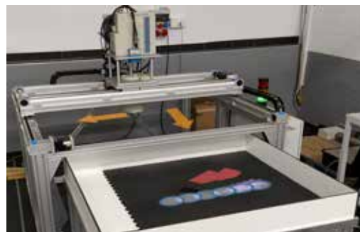
Example of measuring table for spatially resolving radiological emissions
