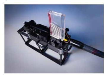
Another innovation in the plugging process is a rapid plug loader with several features that increase plugging production rates. The advanced features include a torque-controlled plug locking station, video verification of plug-to-roll position, encoder position and torque feedback for the pusher station.
