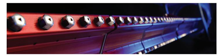
Framatome's water lance system cleans PWR steam generators using a highpressure, high-flow water jet with 90 degree sweeping action for effective sludge removal in square or triangular tube pitches.
