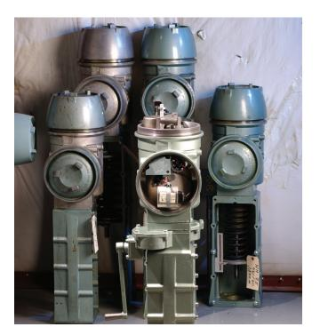
Framatome is the nuclear industry's only ASCO Service Center authorized to overhaul and repair NH90 and AH90 series actuators.
