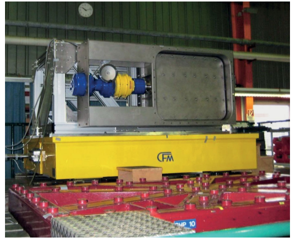
Hydrogen Mixing Damper during seismic tests at Framatome's test bench
