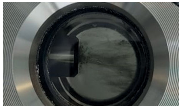
H 2 injected via nozzle into water at 190 bar
