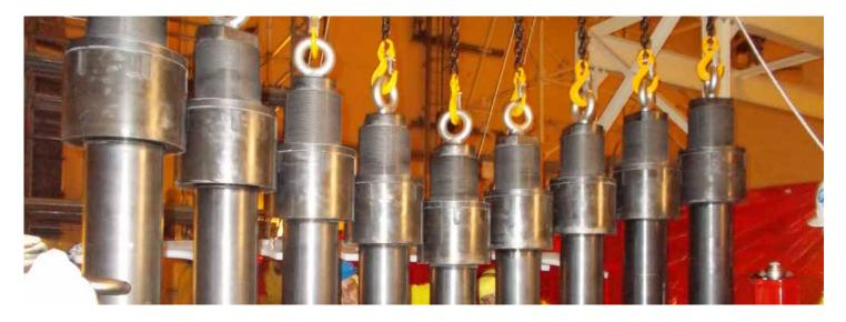
Framatome delivers a multi-stud handling system, designed to remove multiple studs from the reactor head simultaneously. This design can be modified to accept a wide variety of head and stud diameters as well as quantity of studs.
