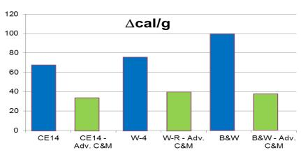
With the AREA methodology the impact of the control rod ejection event is greatly reduced. Enthalpy deposition rates are effectively half of those assessed by legacy analysis. The margin created by this advanced analysis process removes Control Rod Ejection from the list of limiting events for all plant types evaluated to date.
