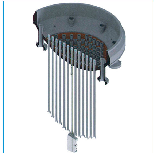
Schematic snap of a BWR-calotte and control rod drive nozzles. The RIS (Rod Internal Segmenter) is inserted from below, cutting the nozzles closely to the calotte.
