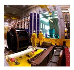
The Pump & Motor Service Center provides inspection, repair, refurbishment and specialized resources to extend the life of critical plant components including pumps, motors and seals.
