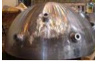
Pressurizer bottom Head
