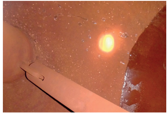
Effect of FFA on condenser floor (low wettability)
