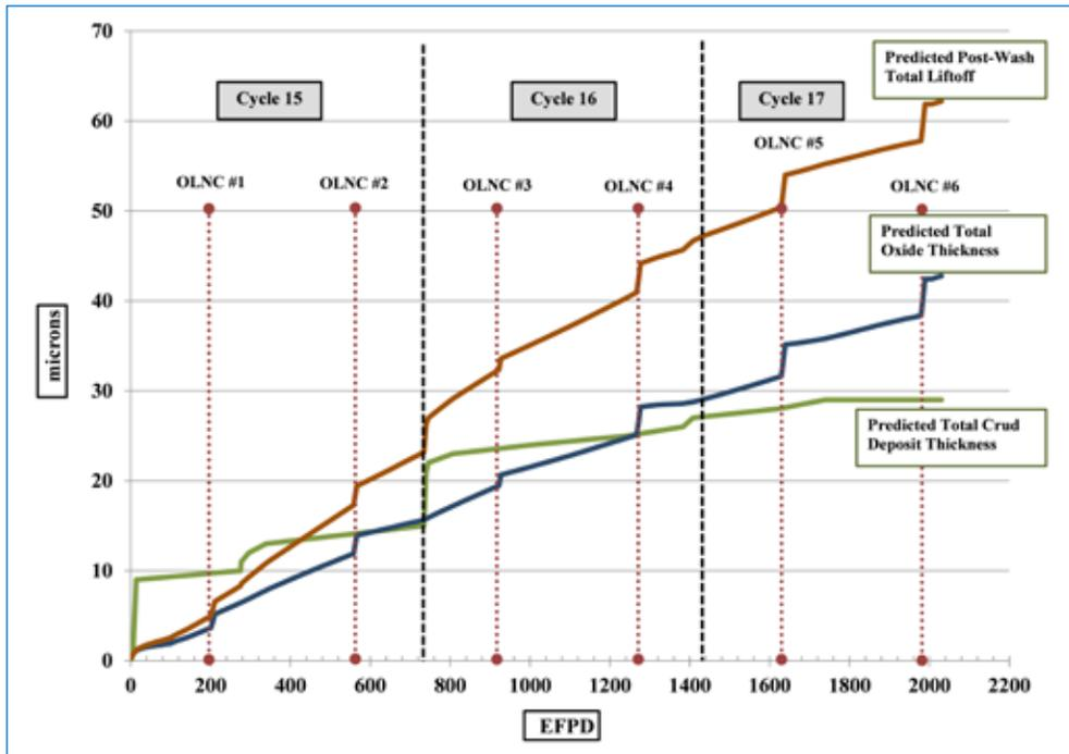
Figure 1: Predicted post-washing total liftoff at limiting core location
