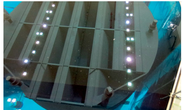
Steam dryer before decontamination: under water storage necessary
