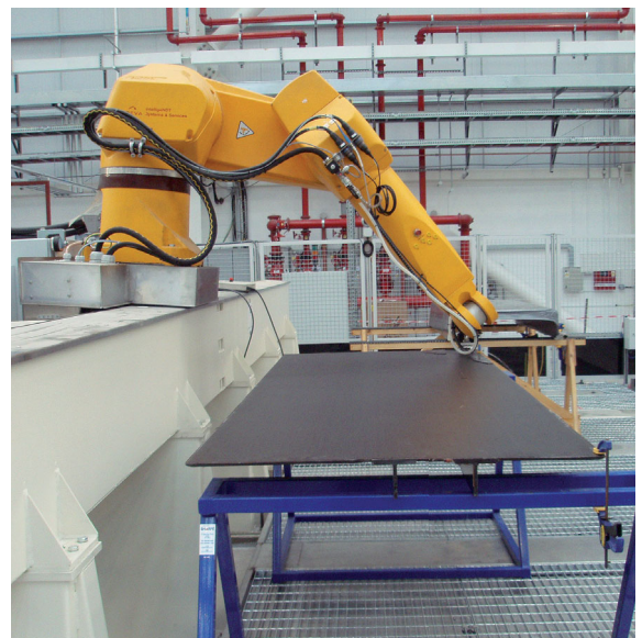
Mono Robot System on rail for an increased inspection volume
