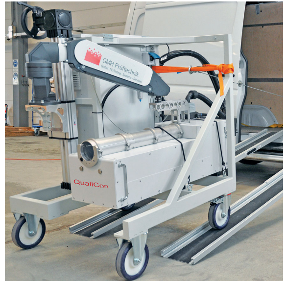
Loading of the mobile ultrasonic inspection system
