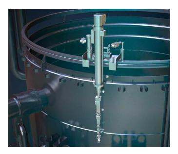
The HawkEye Visual Inspection Manipulator operates on a standard ring platform and performs visual examinations in parallel with shroud UT examinations. It delivers video cameras to target examination areas with full-position feedback integrated into the video record.
