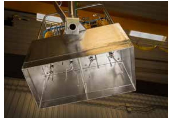
Bottom view of sipping hood showing telescoping sample nozzles for eight fuel assembly positions
