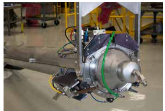
Sipping canister shown with handling bail and lid configuration in closed position
