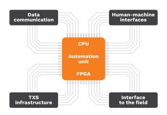
Virtually every element of the safety I&C system architecture is implemented by combining sets of CPU-based TELEPERM XS automation computers and/or FPGA-based automation units in network structures. This meets all requirements for redundancy, physical separation and equipment diversity. Gateways with standard industrial protocols ease interfacing to process computers or third-party control systems.
