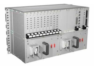
An advanced cabinet cooling concept extends the range of supported room temperatures, internal cabinet temperature monitoring and automatic fan speed adjustment.
