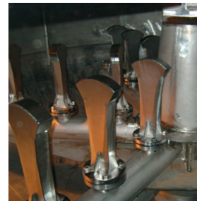
Example of Stage 1 Venturi Scrubber
