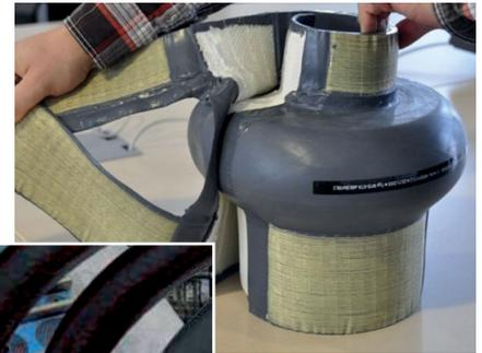
Silicone sleeve for pipe wall penetrations
