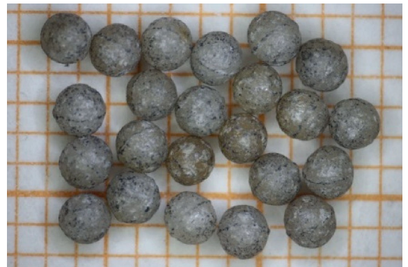
Sintered NAS targets (boxes measure 1 mm)
