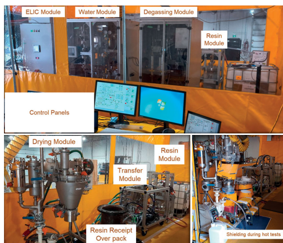
Set-up of a test facility for radioactive resin waste
