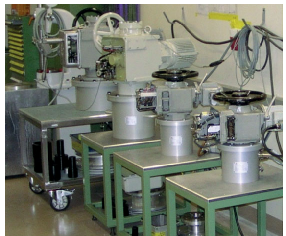
Electro-mechanic brakes with different measurement ranges
