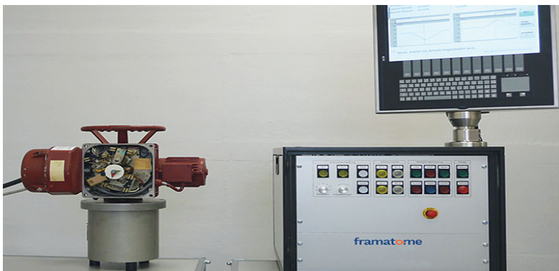
ATESY - Actuator Test System
