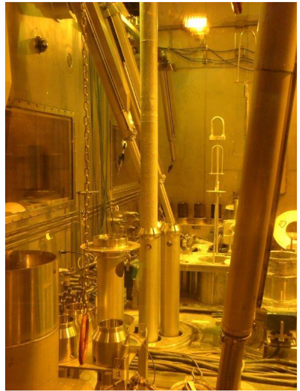
Remote handling in the hot cell for the Super-Phenix Fitting an adapter on a lateral neutron shield
