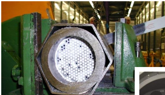
Dismantling of dummy core assemblies (Super-Phenix)
