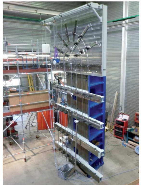
SOPHIE bench: vibration of steam generator tubes
