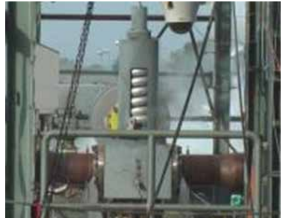
Pressure relief valve on test bench
