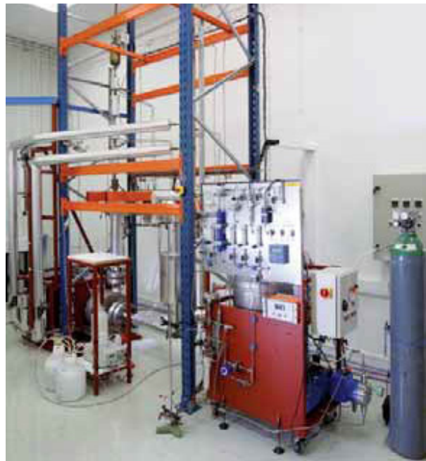
EMILIE test loop – parametric studies of secondary side steam generator clogging
