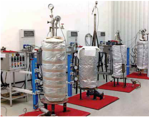
Static autoclaves, fully instrumented for aqueous corrosion testing of all kinds of materials at high temperature under primary and secondary side conditions
