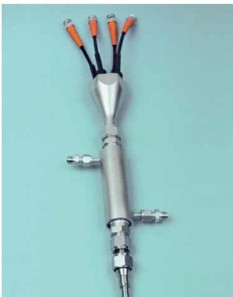
Laboratory version of the high-temperature reference electrode
