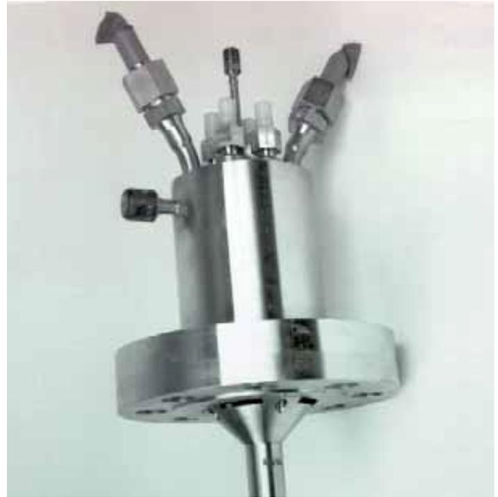
Flange version of the high-temperature reference electrode
