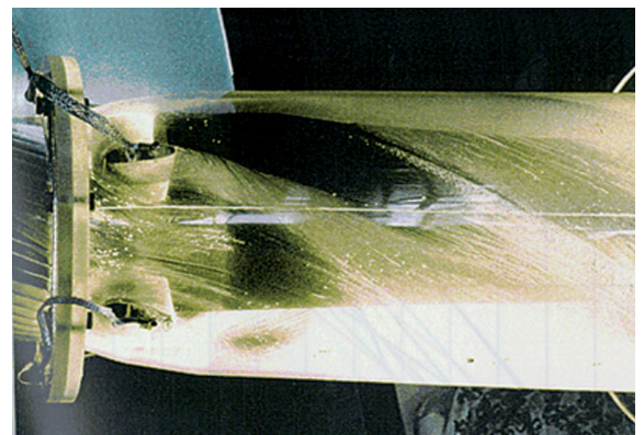
Simulation of swirling gas turbine exit flow for studies related to heat recovery steam generators
