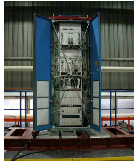
I&C cabinet qualification tests
