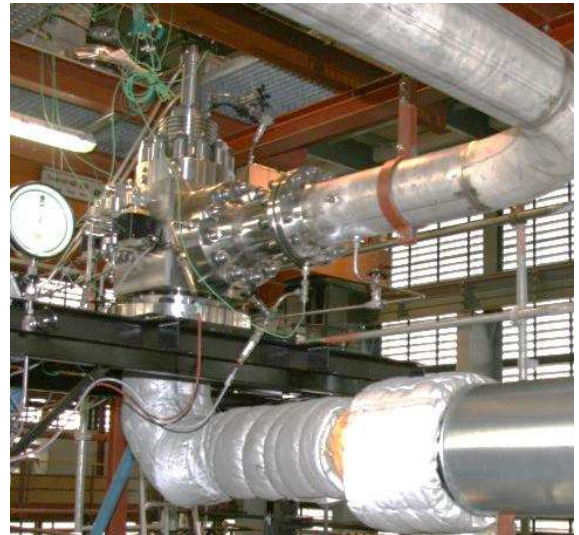
Functional test of a safety valve under operational and accident conditions on open test loop
